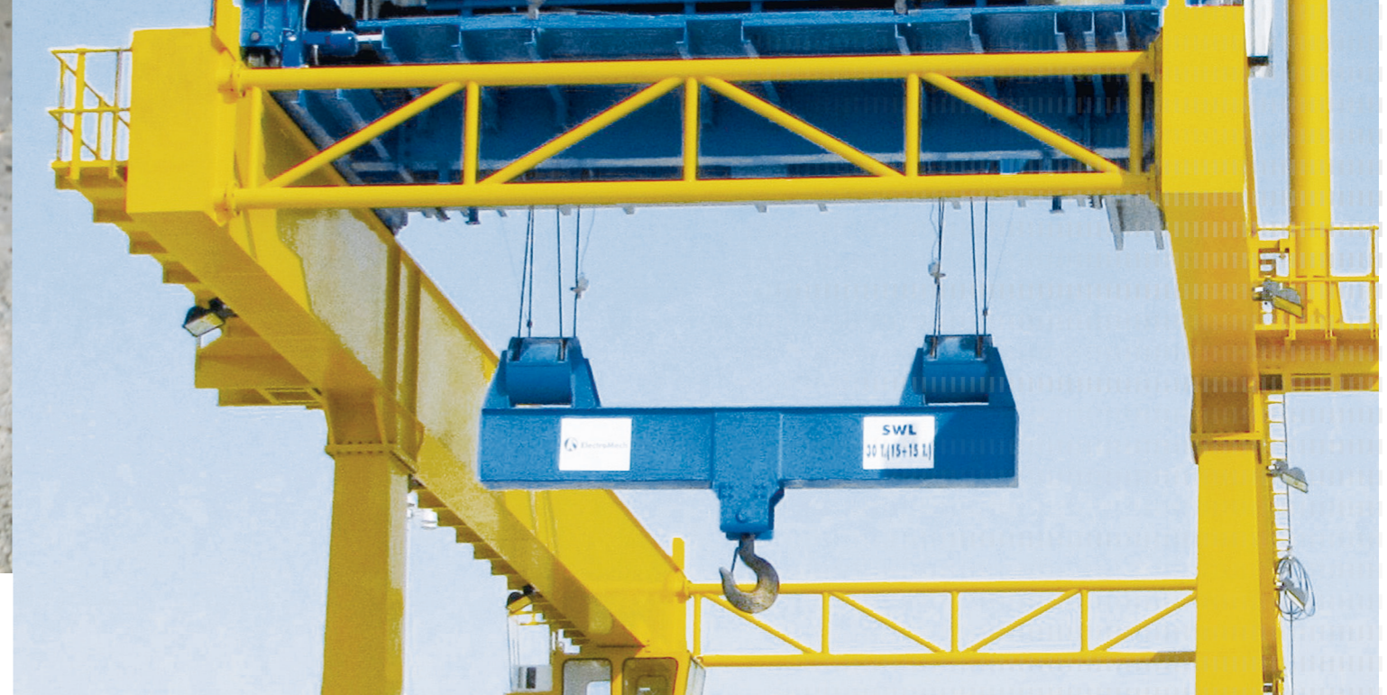
In the island city of Abu Dhabi, new sewage tunnels are bored up to 100 m below the sprawling metropolis. Robust NORD drives in synchronized operation enable hoist systems to take utility platforms safely down deep-reaching access shafts and up again.
