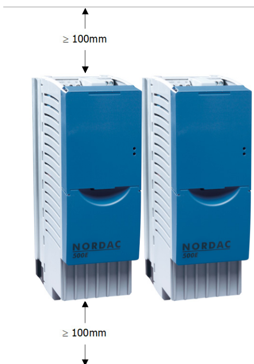
Fig. 1 Mounting distances for SK 5xxE
