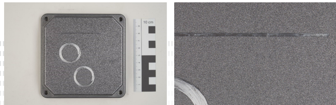
Picture after Salt spray test of 720 h, scribe made before beginning, pull-of test performed after test completion
