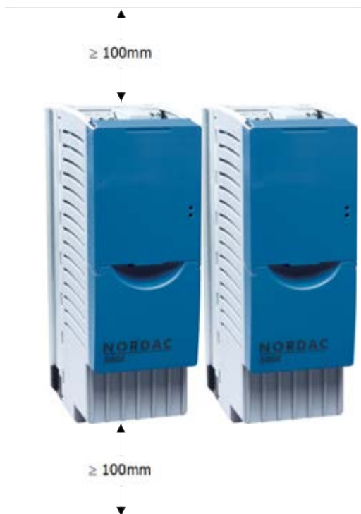
Illustration 1: Distances de montage SK 5xxE
