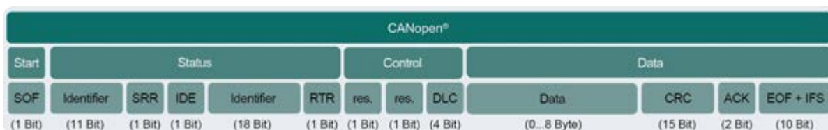
Abbildung 4: CANopen-Extended-Frame – 29-Bit-Identifier
