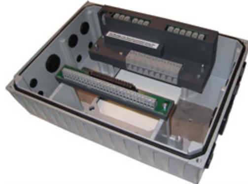
Figure 3: Connection unit size 4
